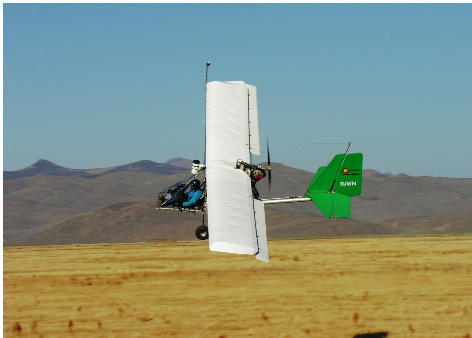
Survey aircraft - magnetic sensor is mounted on the right wing.
